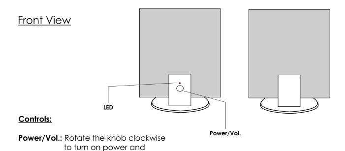
**LED Display:** Indicates system on/off.
